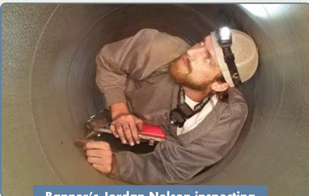
Banner's Jordan Nelson inspecting interior of 24-inch steel pipe
