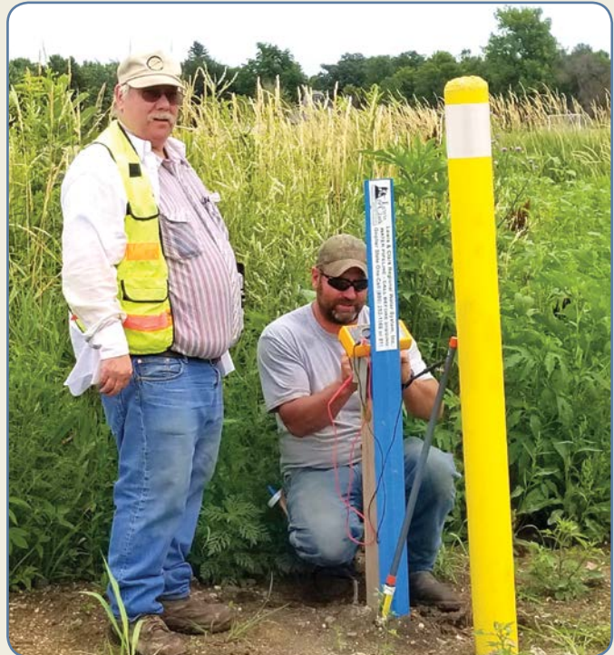
Distribution Operator Jay Nelson (right) and Bill Spickelmire from RustNot, Banner's corrosion consultant, testing the continuity of the tracer wires on the pipeline between Adrian and Worthington. Tracer wires are used whenever the pipe needs to be located.
