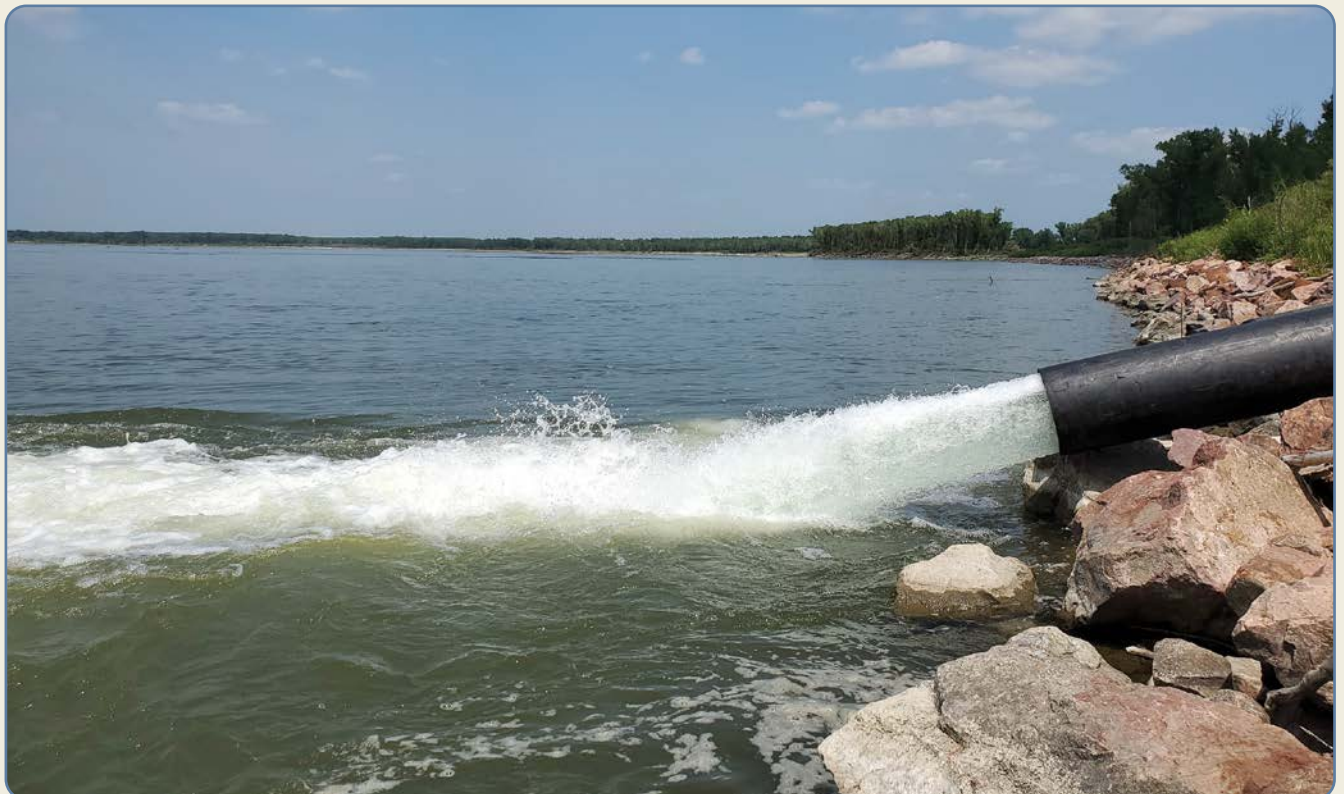
Data from the Site B collector well pump test is being used by SDGS in their analysis of how much of the well water is induced from the river
