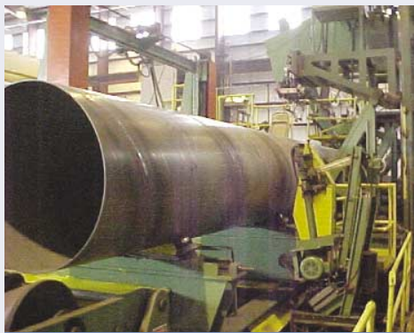
Lewis & Clark's 48" steel pipe being fabricated and welded in South Carolina
