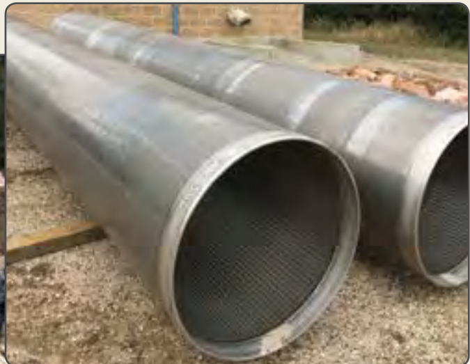
Above: 36 inch diameter screen used for the replacement well
